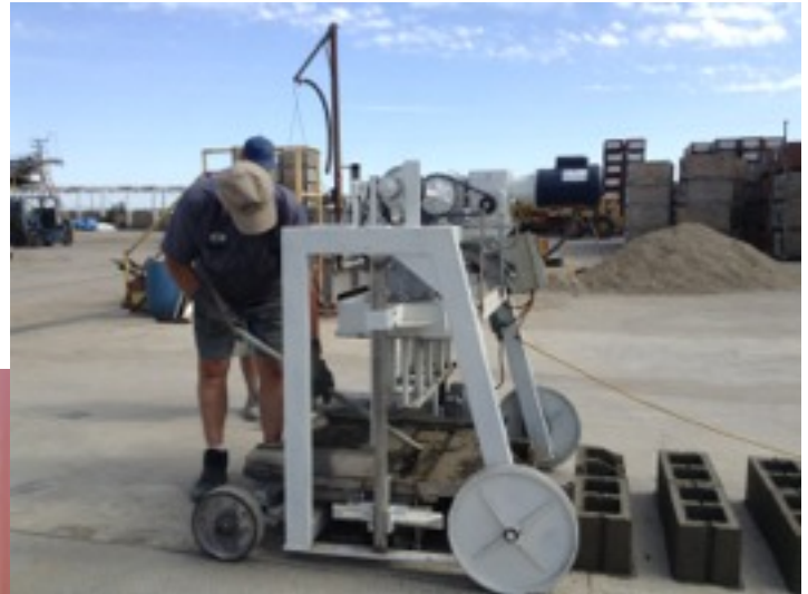
Testing the block making machine before shipping. Can do about 400 per day.
